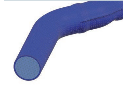
Boundary layer mesh of an automotive exhaust.
